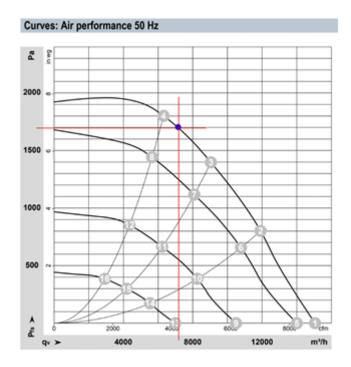
The maximum achievable static pressure at 2m3/s will be circa 1700Pa. Any additional system pressure will result in a loss of volume as the duty point travels left along the full speed curve.
