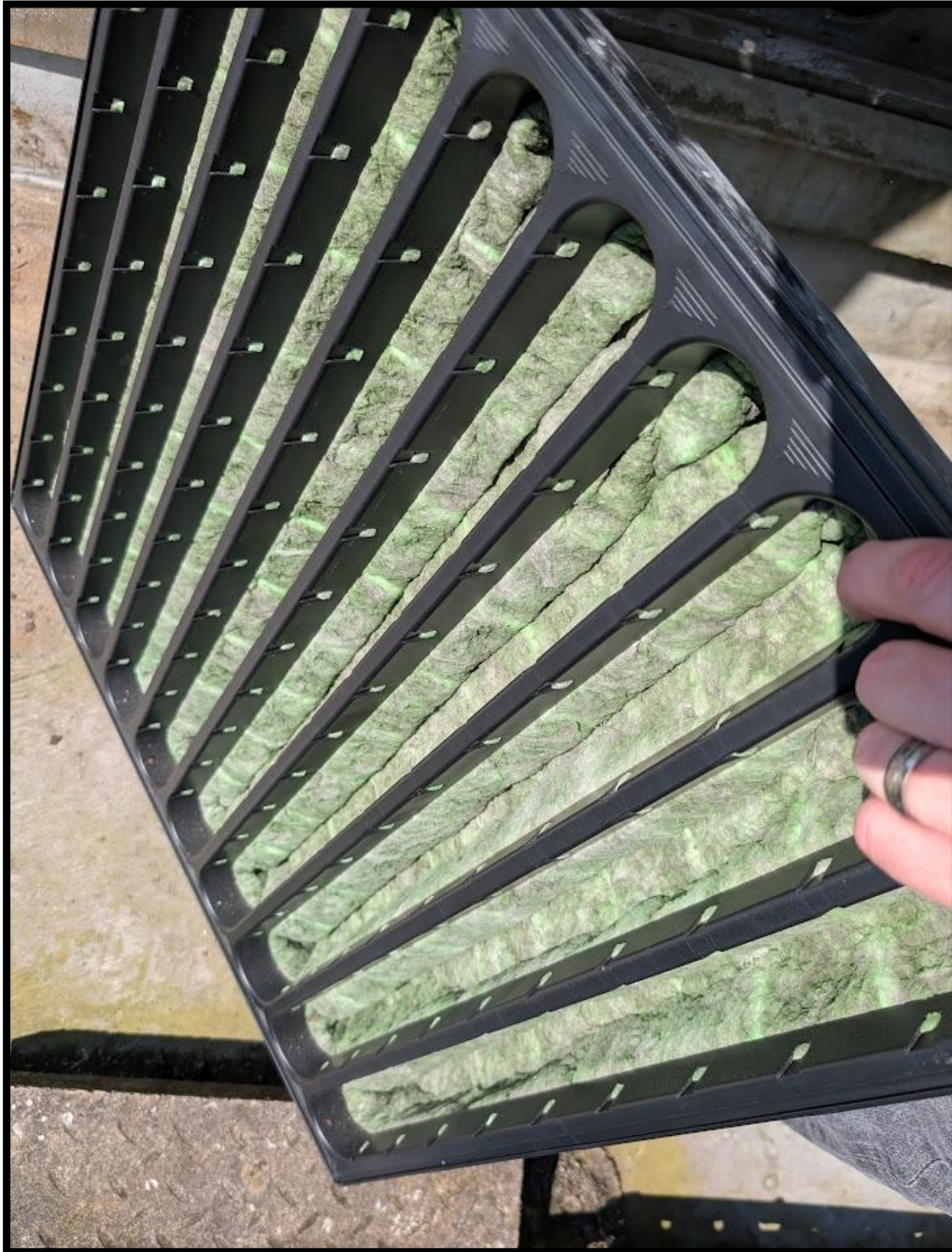
Signs of Water Logging in Bag Filters
